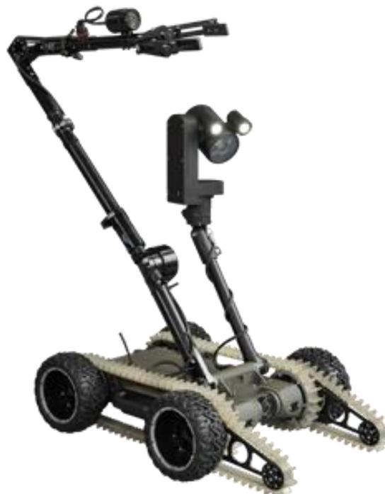
Equipped with its specific drives, the robot efficiently travels across uneven terrain and obstacles with the inclination as high as 45°. The robot wheels are easily removed in case of the need to further reduce the robot's overall dimensions. Small weight and compact size enable convenient transportation, possibly in a backpack.
