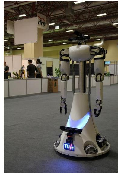
**Figure 2.1: Picture of service robot AMIGO, developed by TUE.**
