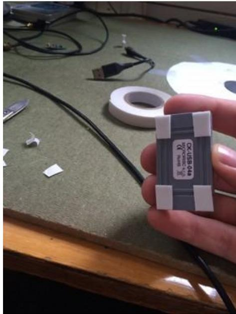
*Figure 8. IQRF programmer with a double sided scotch*
